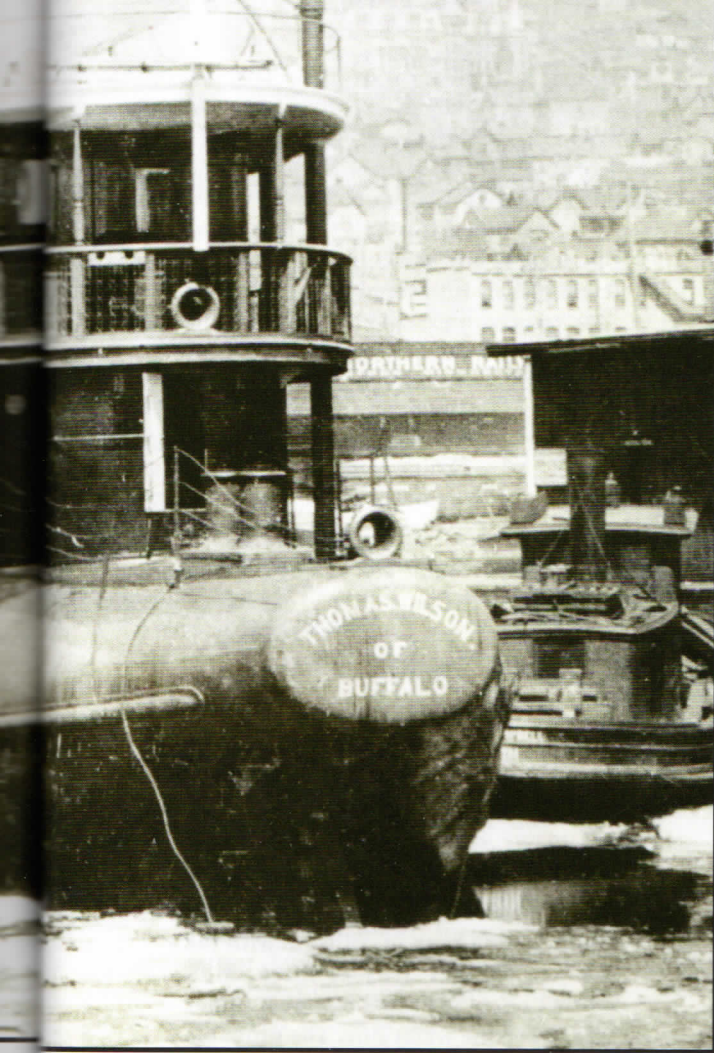
Right Top Corner: The rounded steel sheets of a whaleback's hull easily rolled or pushed lake ice out of the way. (Kohl-Forsberg Archives)
